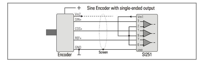
When the reference signals REF+ and REF- are not used or not available, the related inputs of the converter must be tied to a defined potential.
