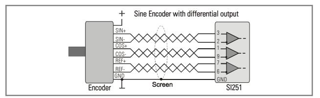
With sensors using single-ended outputs, the sensor signals SIN, COS and REF are connected to the corresponding input pins. The inverted inputs of the unit are tied to <u>either</u> the mean voltage output Vm (pin 8) of the unit, or to a corresponding voltage reference of the sensor itself
