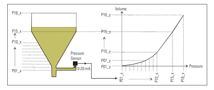
To solve the problem, we divide the non-linear part of the tank into 14 parts. We enter the expected display values of the pressure sensor to registers P01\_x to P15\_x.
