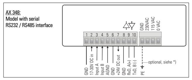
\*) The connection of PE is optional and not necessary for safety or for EMC.
