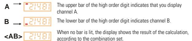
When you use one of the combined modes, you will first have to do the same settings as with the "Dual" mode for individual display of inputs A and B.
