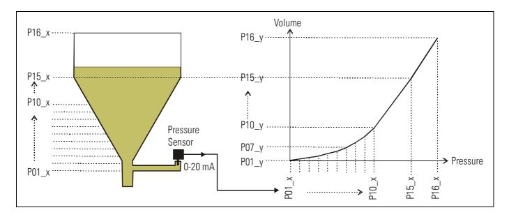
To solve the problem, we divide the non-linear part of the tank into 14 parts. We enter the expected display values of the pressure sensor to registers P01\_x to P15\_x. For the linear part of the tank it is sufficient to store the final pressure value to register P16\_x. Now we can easily calculate the appropriate filling quantities and enter these values to the registers P01\_y to P16\_y.
