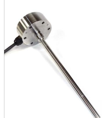
The GYAF-probe is an all-in-one type flat-head with integrated controller. After supplying DC 24V an analogue voltage or current signal is obtained. The flange type offers easy mount and short additional length.
